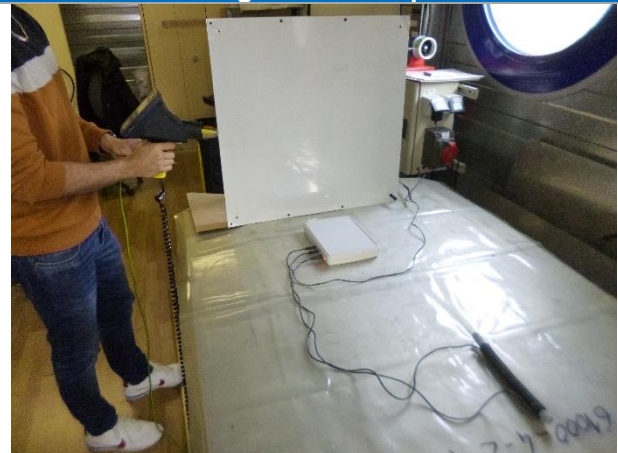
Electrostatic discharges - Indirect contact discharges – VCP1 left face
